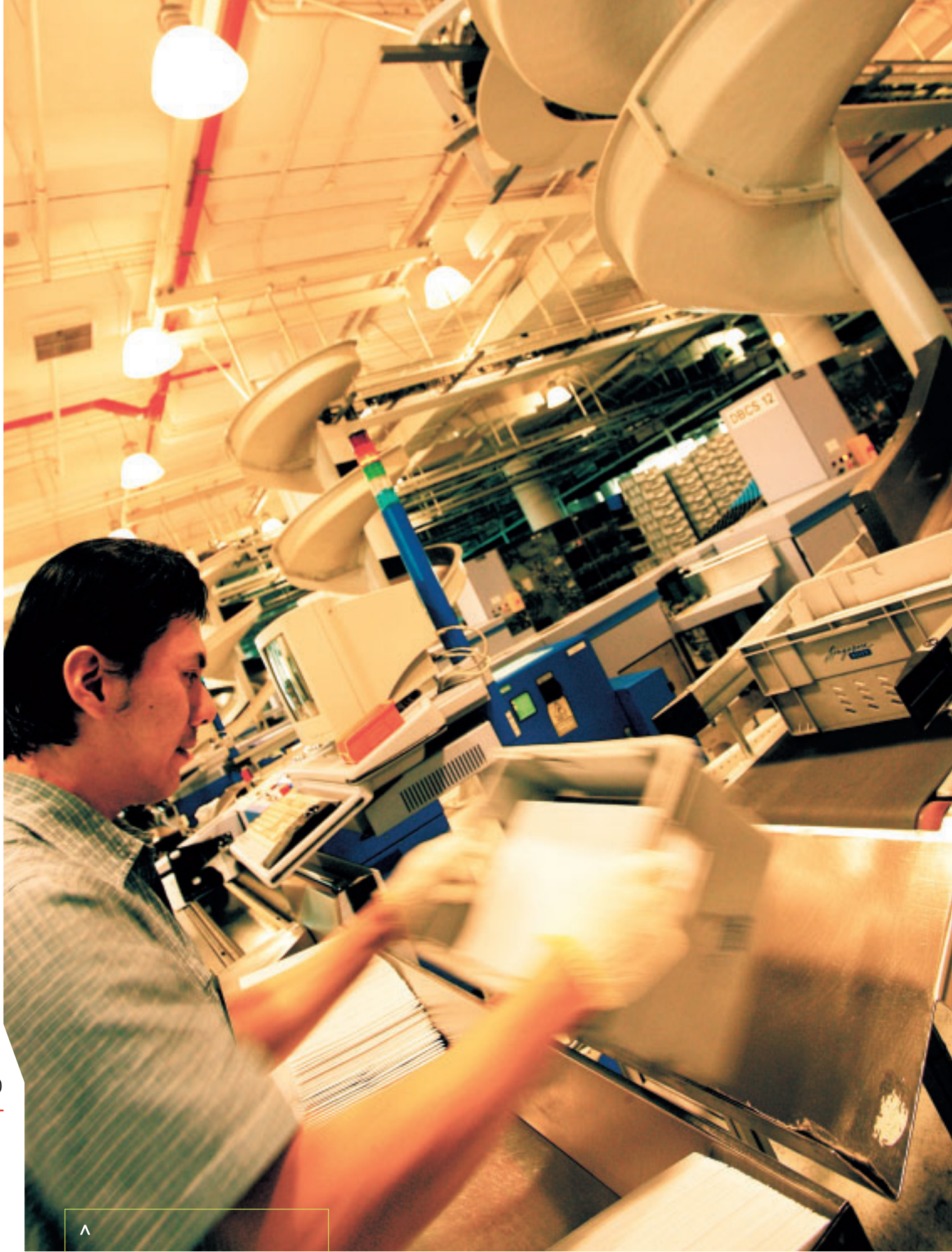
Trays of preprocessed mail arrive at the Delivery Barcode Sorter machine to be sorted to delivery sequence before despatch.
