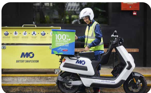
Trial of electric motorbikes with swappable batteries
